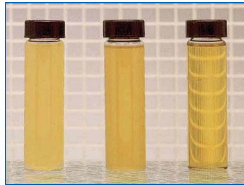
Free water removal in typical turbine oil: bright clear aspect shows absence of free water
